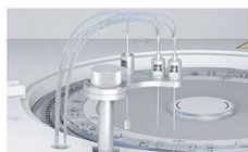
Washing Probe Independent 3-step washing system.
